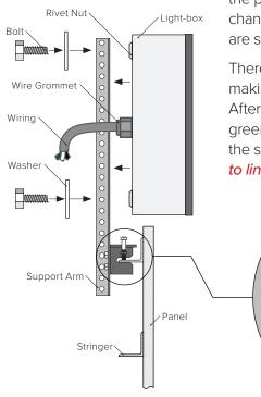
The prop can install directly to the face of the panel with washers and bolts or above the panel using Support Arms for structural support allowing for billboard vinyl copy changes without removing the light-boxes. Custom tailored installation instructions are sent with every order to match the artwork.
